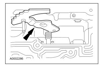
9. Assemble the manual valve inner lever and parking lever actuating rod as shown.
